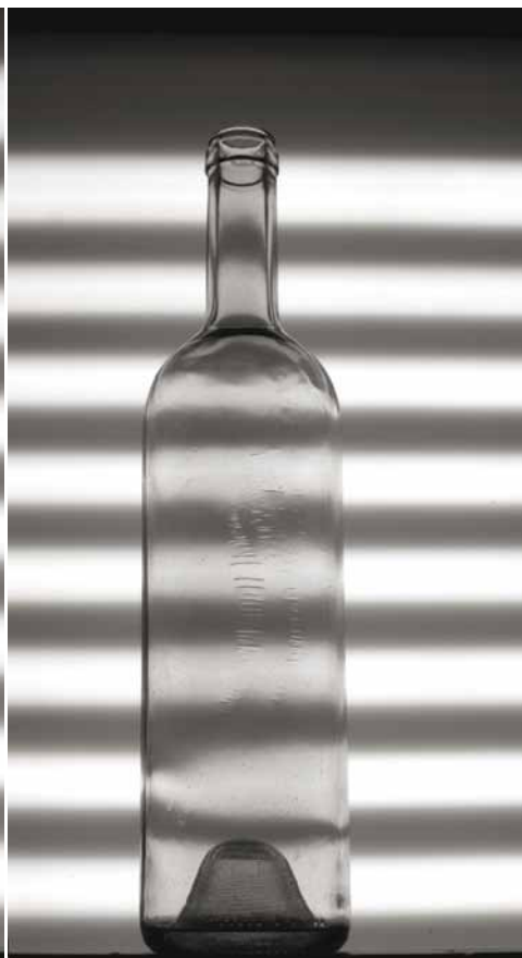
Washboards detected by the Low Contrast detection on a blow & blow container
