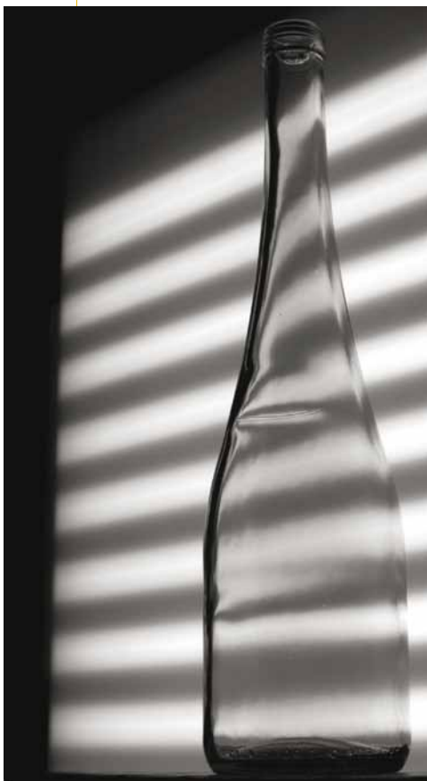
Fold detected by the Low Contrast detection on a blow & blow container
