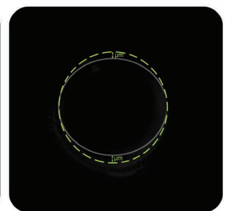
SADDLE defect measurement
