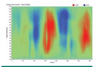
This example shows the glass thickness distribution on the sidewall of a bottle. The X axis shows the radial position in degrees around the bottle whereas the Y axis show the height location on the side wall. Red denotes thinner glass, blue thicker glass and green is the optimum thickness.
