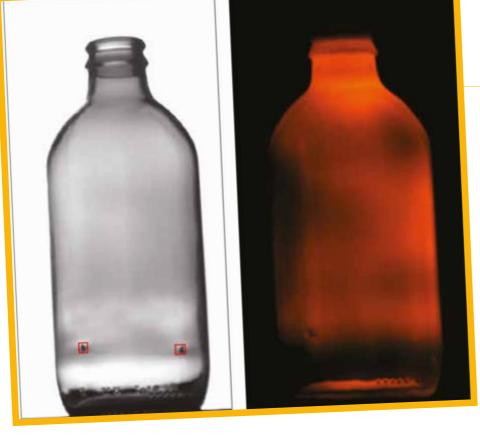
at the hot-end. The high-definition matrix cameras and measurement by transmission both achieve an excellent defect detection level compared to infrared camera technology. Infrared images have areas with different brightness levels creating very dark or very bright areas where it makes it impossible to detect defects. The Tiama HOT eve is not impacted by these differences in radiation - which allows for complete inspection of the article from bottom to finish.
