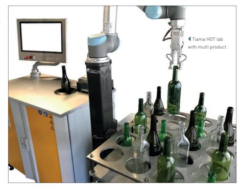
an assortment of bottles, varying in height, shape and diameter into the loading cart. The robot then finds, collects and places the bottles into the Tiama HOT lab one by one and measures them all.
